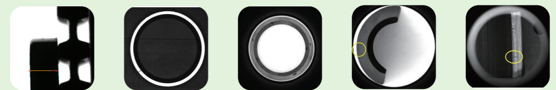
尺寸测量 Dimensional Measurement 倒角 Chamfer 外侧圆周及内倒角测量 Measure Cylindrical Circumference & Inner Chamfer 磁材 Magnetic Material 端面伤 Marks On End
